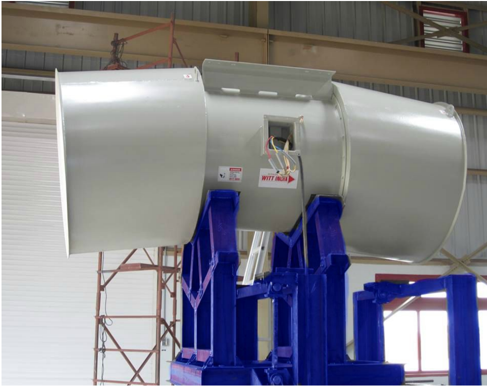
THRUST TEST RIG as per ISO 13350
